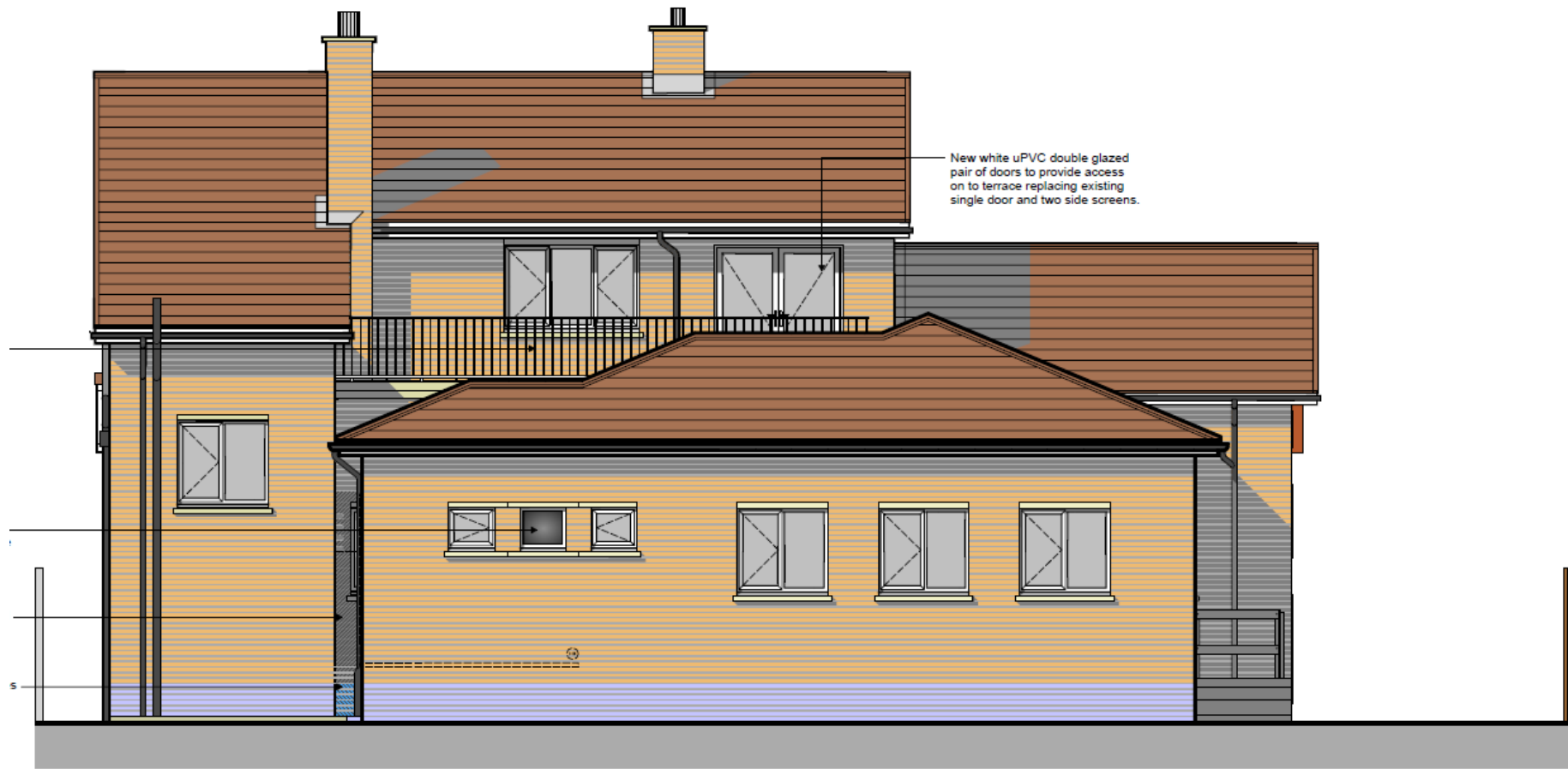
Proposed Rear South Elevation (scale 1:50)
